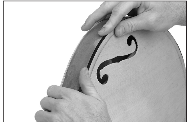
Figure 13. Attaching the binding.
