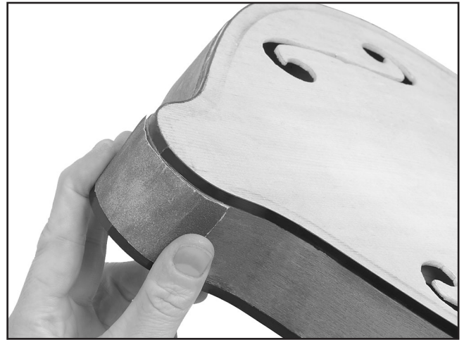
Figure 16. Adjusting the fit of the neck.
