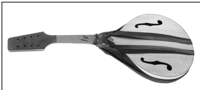
Figure 22. Example of gluing the neck.
