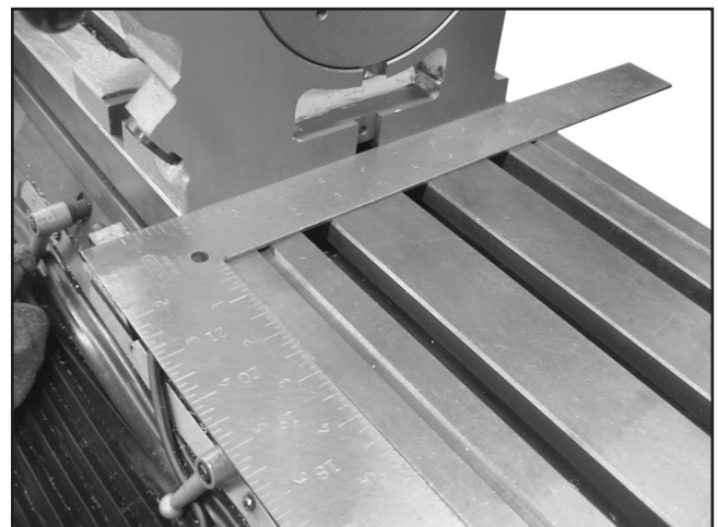
Figure 4. Using a precision square to align the rotary table with the mill table.
