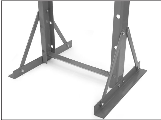
Figure 3. Base supports installed.
