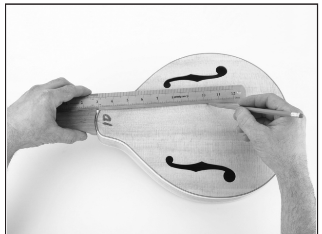
Figure 5. Checking neck alignment.
