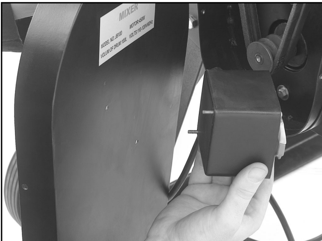
Figure 16. Attaching switch box to the outside pulley with the existing screws in the switch box.
