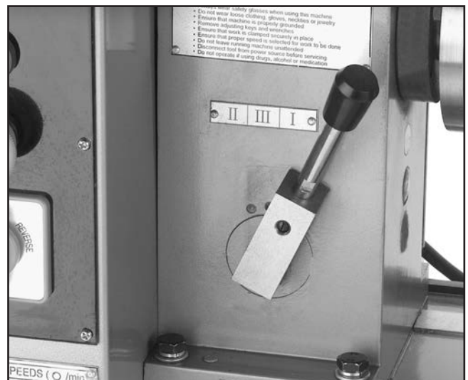
Figure 50. Feed rate lever set to I for 5 TPI.
