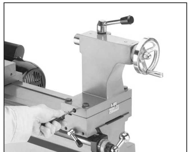
Figure 25. Tailstock offset adjustment screw.
