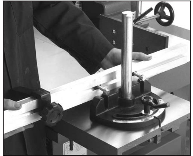
Figure 24. Installing the miter fence.
