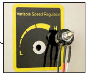
Figure 8. Variable speed dial wiring.
