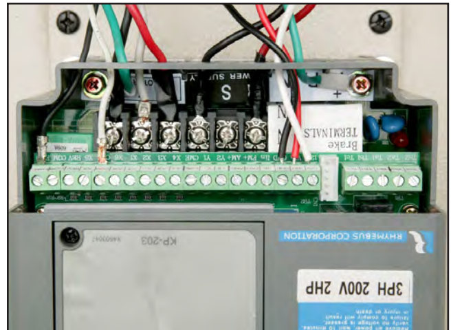
Figure 61. Inverter/Controller box wiring (see wiring diagram on Page 47).
