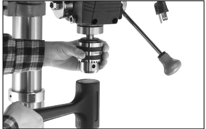
Figure 23. Seating chuck into spindle. (Note retracted jaws.)
