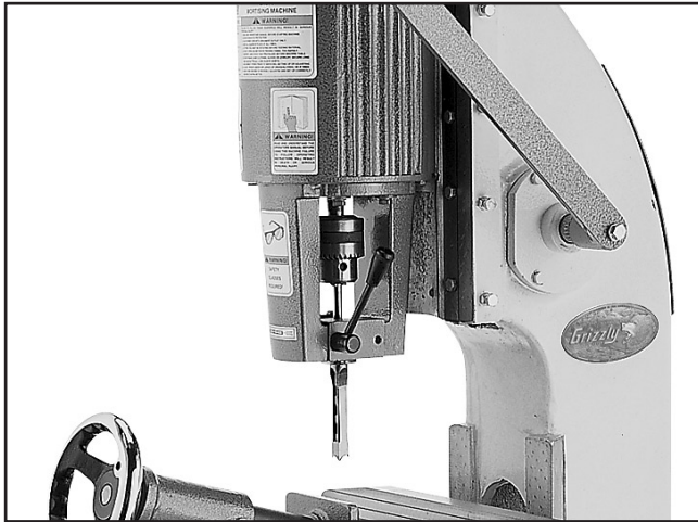
Figure 18. Auger bit and chisel correctly installed.
