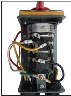
Figure 47. Speed switch wiring.
