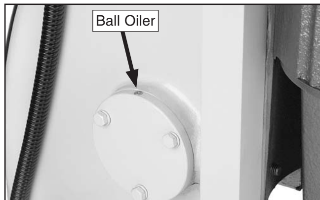
Figure 41. Operating handle pivot (left side).
