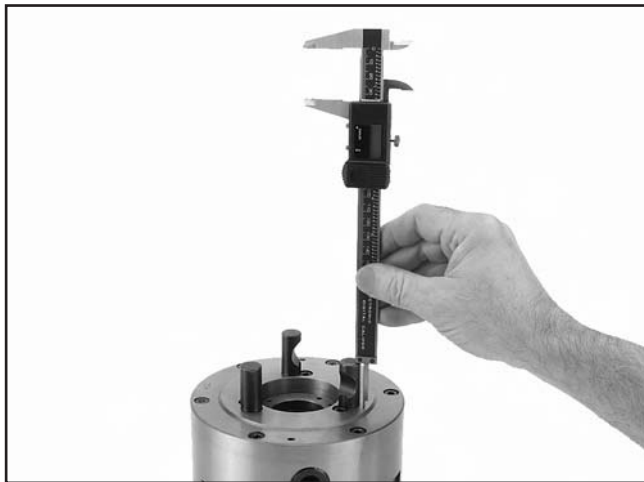
Figure 19. Measuring height of cam-lock studs.
