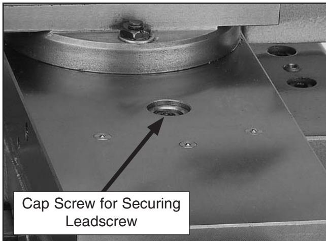
Figure 82. Cap screw securing the leadscrew.
