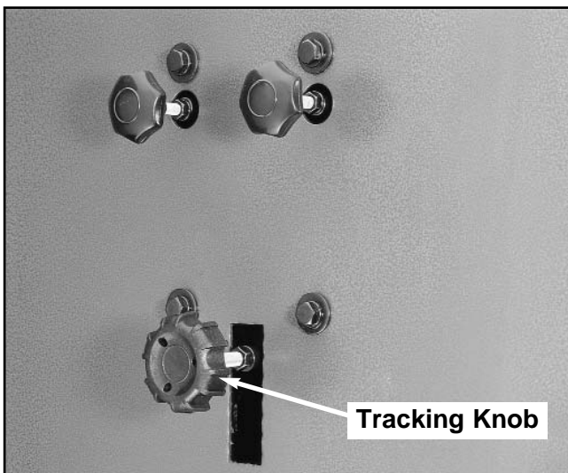
Figure 3. Tracking knob adjustment location.
