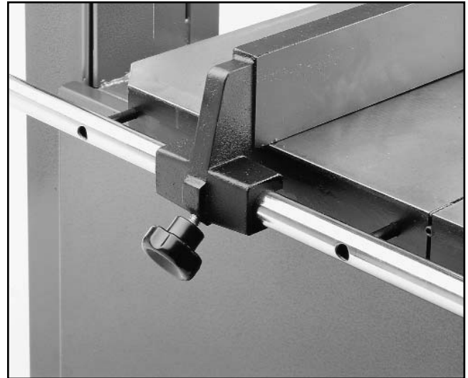
Figure 2. Front rail in place and fence installed.
