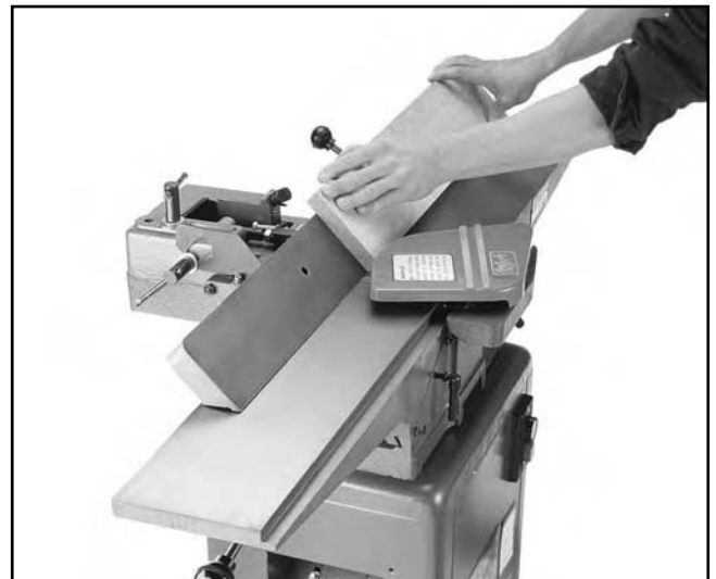
Figure 26. Fence position for bevel jointing.
