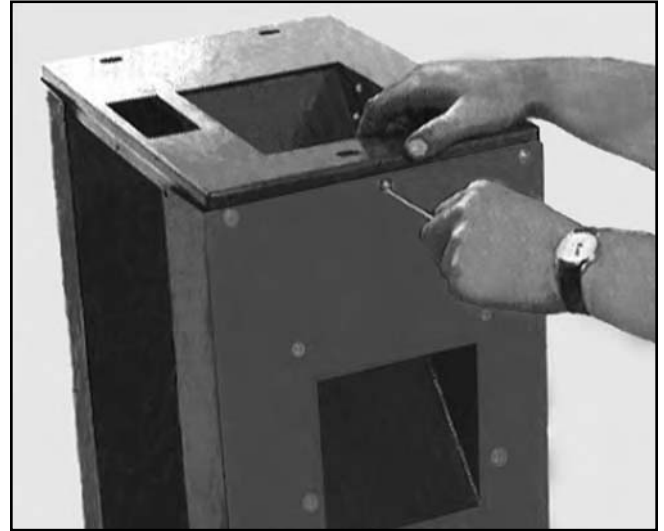
Figure 6. Attaching the top of the stand.
