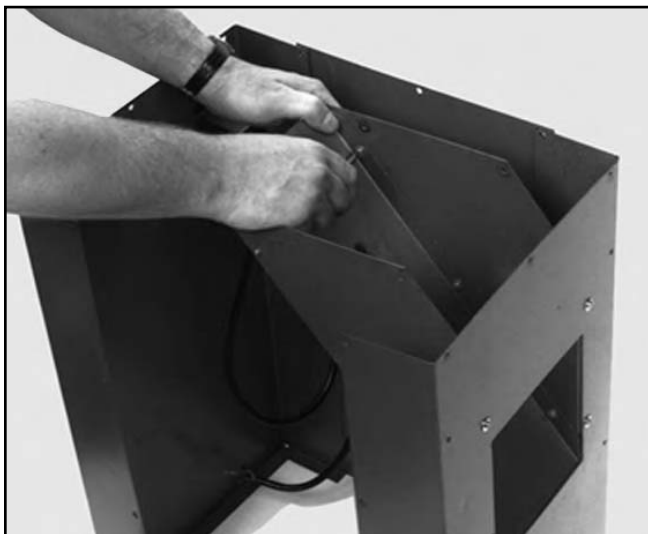
Figure 5. Attaching the dust chute base.
