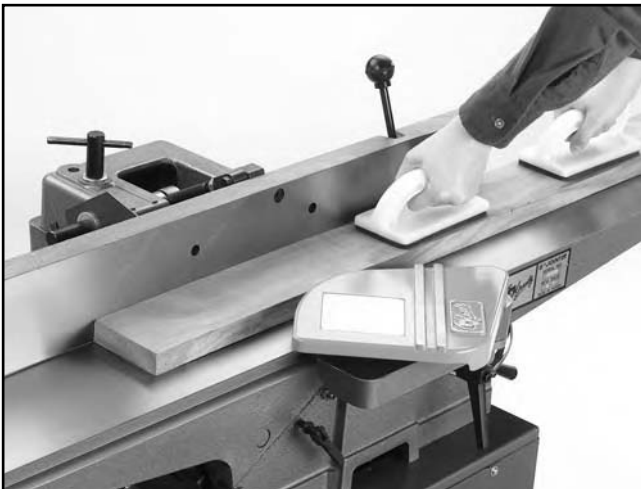
Figure 27. Correct method for surface planing.
