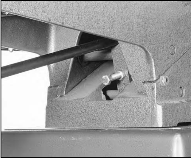
Figure 17. Table stop bolt and check nut.
