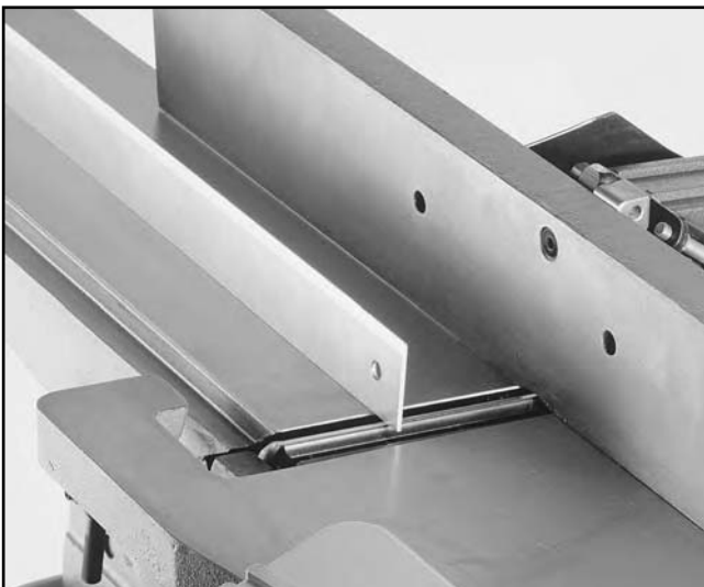
Figure 18. Illustrates the use of a straightedge to ensure proper outfeed adjustment.
