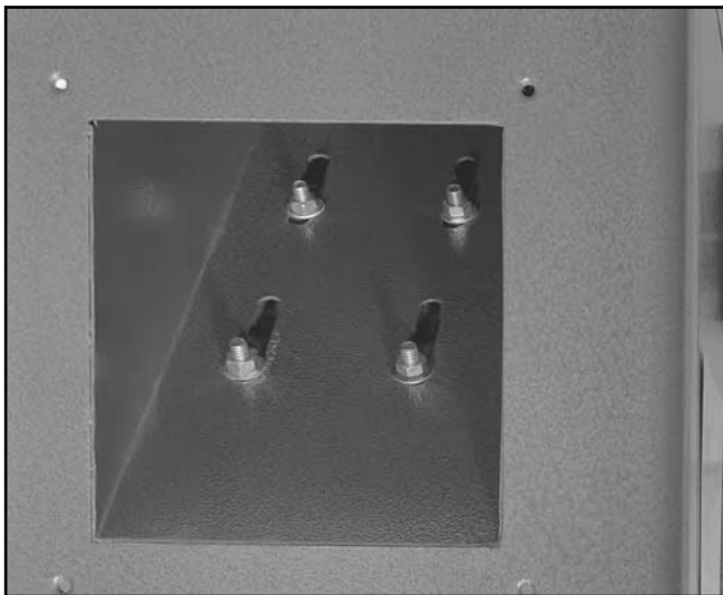
Figure 8. Motor mounts inside dust chute.
