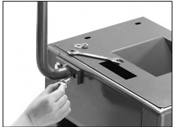
Figure 13A. Mounting pedestal switch to stand.
