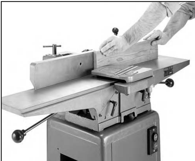
Figure 25. Operator position for edge joining.
