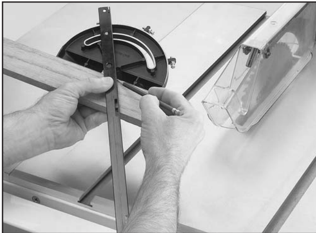
Figure 44. Marking miter line.
