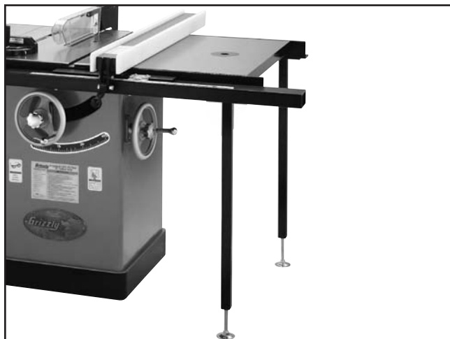
Figure 18. Router table and legs installed.
