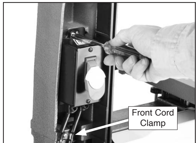
Figure 16. Attaching the switch.
