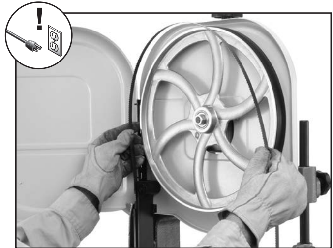
Figure 47. Placing blade on the wheels.
