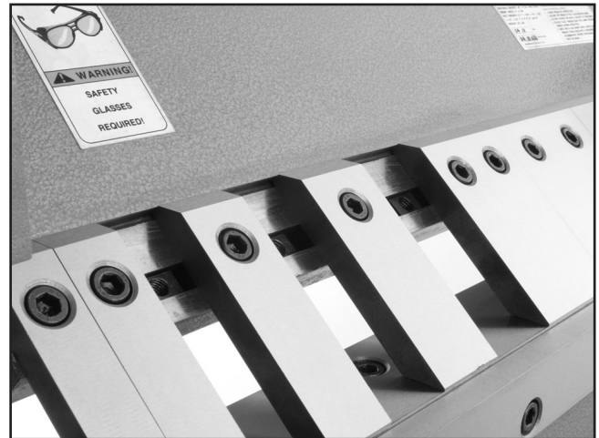
Figure 19. Fingers removed to provide space for matching fingers with box or pan widths.
