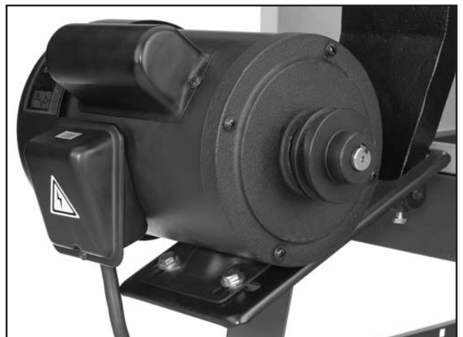
Figure 15. Motor installed on motor plate.
