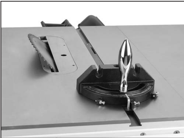
Figure 40. Blade tilted to 45° (guard removed for clarity).
