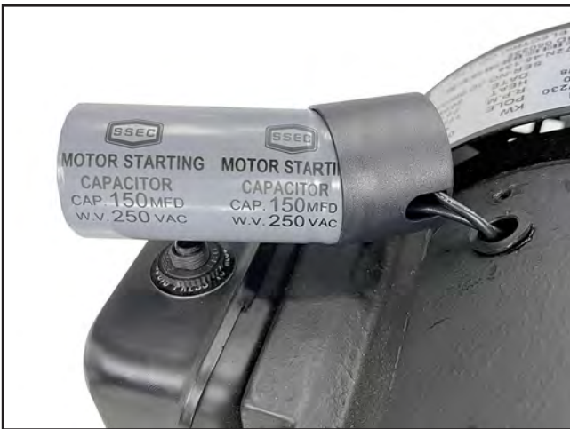
Figure 15. Main motor capacitor wiring.
