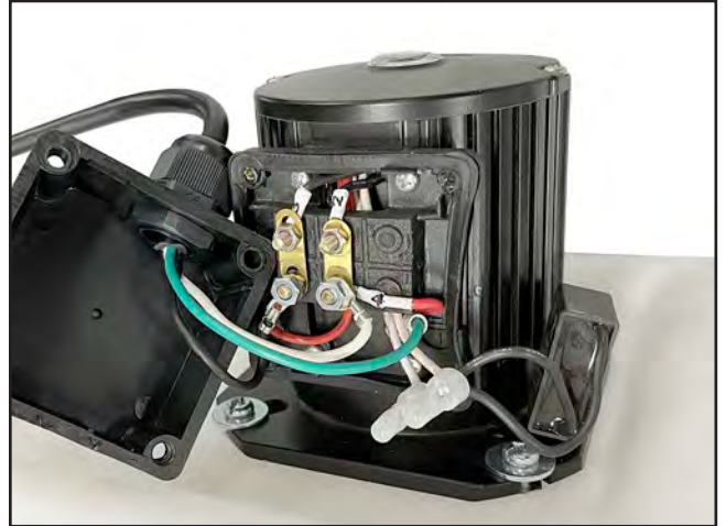
Figure 17. Coolant pump motor wiring (115V).
