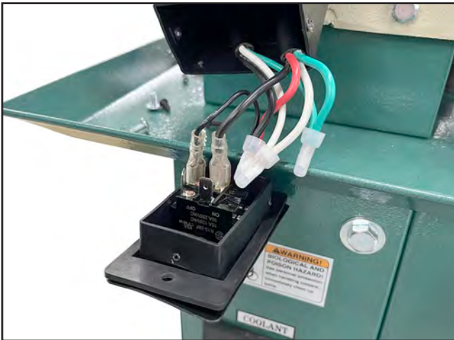
Figure 16. Motor ON/OFF switch wiring.
