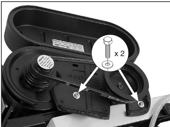
Figure 19. Pulley cover installed.
