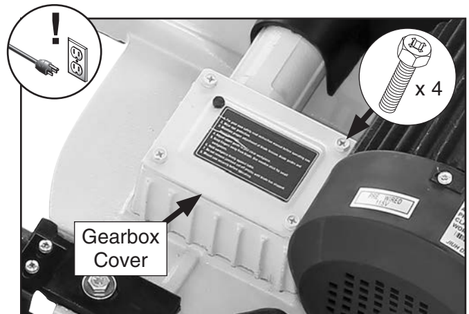
Figure 69. Location of gearbox cover and bolts.
