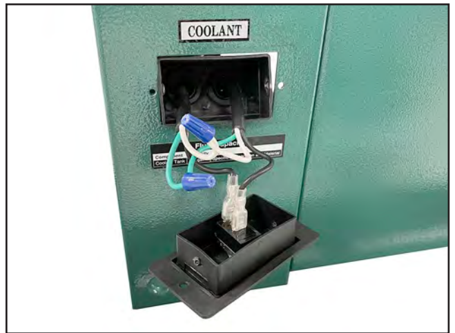
Figure 18. Coolant pump ON/OFF switch wiring.
