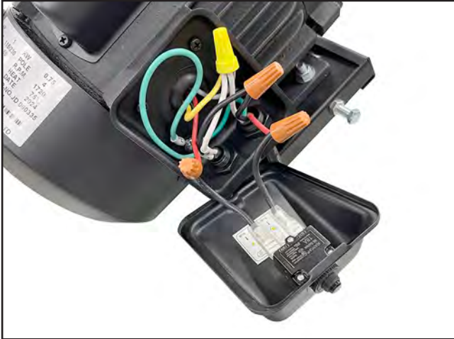
Figure 14. Main motor wiring (115V).
