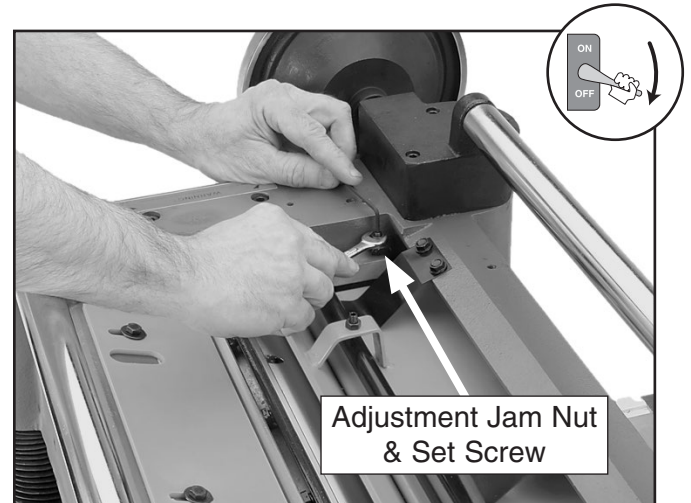
Figure 46. Adjusting the pressure bar height.
