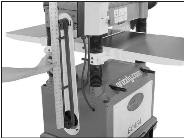
Figure 52. Checking pulley alignment.
