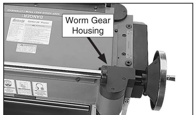
Figure 29. Location of the table height worm gear housing.
